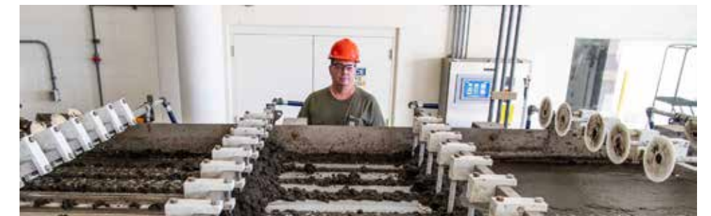
Matt Mink checks biosolids consistency in the gravity belt filter press (Komline-Sanderson) at the Bloomington-Normal Water Reclamation District Southeast plant site.
