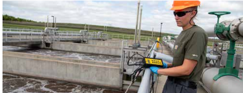
Caitlin Raasch uses a solids meter (YSI, a Xylem brand) to measure mixed liquor suspended solids levels in an aeration basin.
