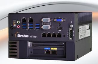
Zero-touch edge computing for up to 10,000 input-output operations (I/Os) in pharma manufacturing, food & beverage, specialty chemicals, oil & gas, and other industrial verticals.
