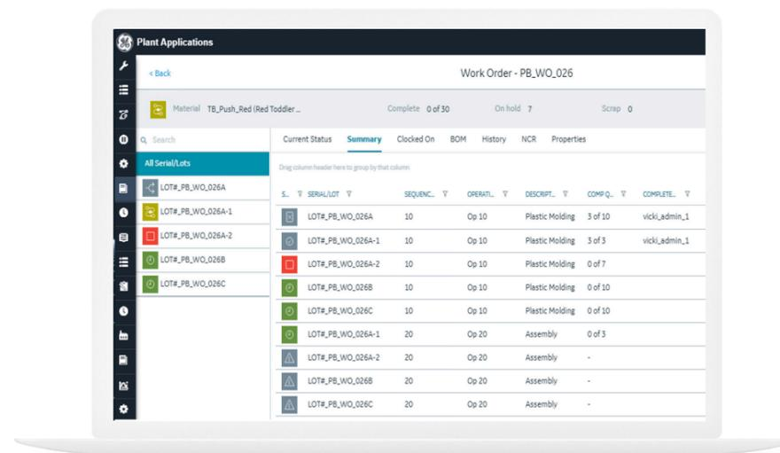
The screenshot displays the Proficy MES interface for a 'Work Order - PB\_WO\_026'. It shows a summary table with columns for 'S.', 'SERIAL/LOT', 'SEQUENC.', 'OPERATL.', 'DESCRPT.', 'COMPQ.', and 'COMPLETE.'. The table lists various production steps, including Plastic Molding and Assembly, with their respective quantities and completion status.
