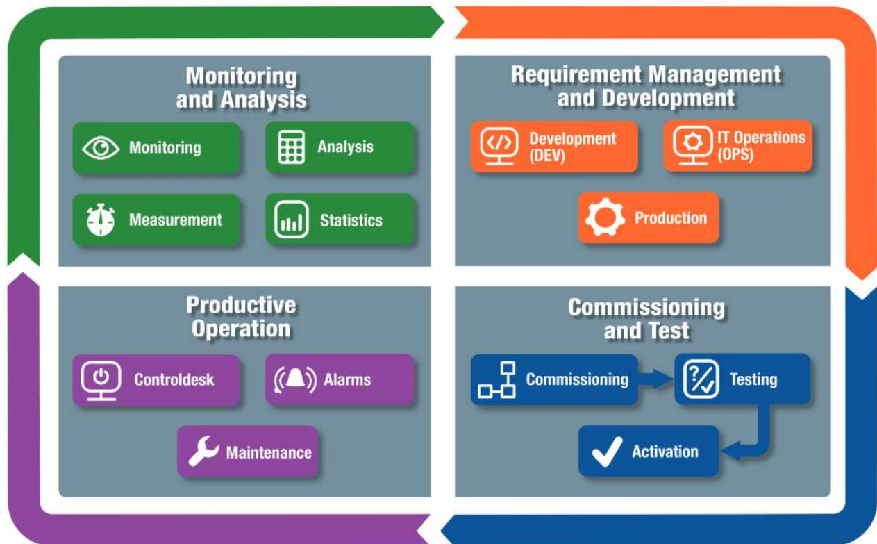
Fig. 1. The continuous adaptation and improvement process of Industrial DevOps
